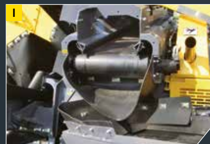
Cross conveyor belts on 3D versions For better screened material flow to the stockpile conveyors.
