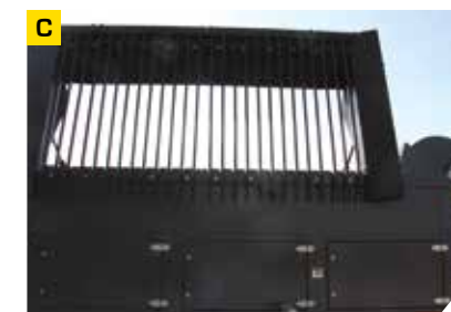
9.2 m³ hopper, long loading lengths Enables you to use wider loading buckets.
