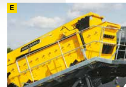
High Energy screenbox Features adjustable inclination, achieves exceptional results with an amplitude of up to 10 mm and the highest capacity even with difficult materials.
