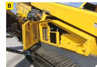
Wide access engine bay doors Provide perfect access for service and maintenance of engine and hydraulics.
