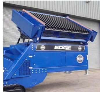
EDGE Innovate's range of feeder stackers have the ability to handle a wide range of applications and capacity requirements. Available with discharge conveyors from 30ft to 90ft, various chassis formats, power-source options and an infinite number of add on options such as a two deck vibrating live head, overband magnet, wireless remote functionality and radio controlled reject grid; the feeder stacker range is arguably EDGE Innovate's most versatile product.
