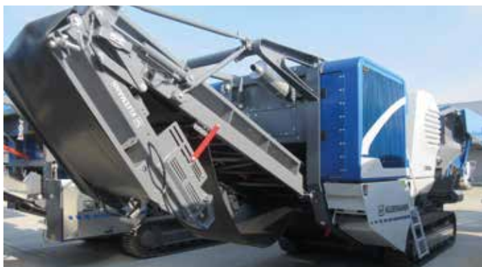
Extended crusher discharge conveyor, foldable for simple transport.
